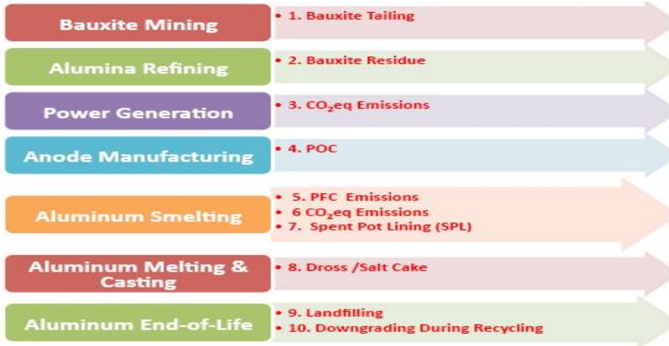
Fig.1: Aluminium production processes/ by product emissions
