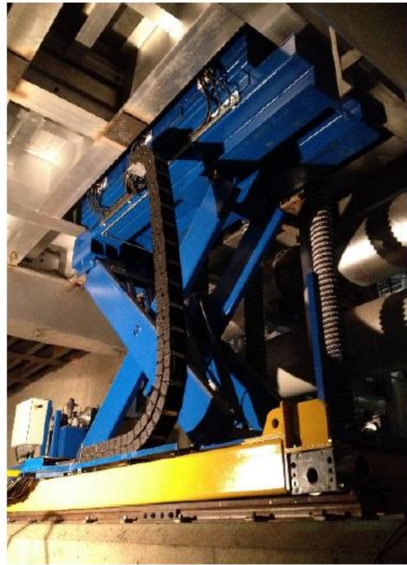
SIBER FORCE® EMS Bottom-mounted with wheels on a support frame with rails (left) and Lift System (right)
