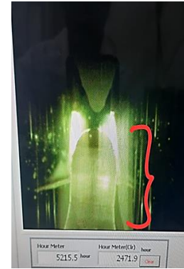
Float Zone growing the crystal from melt
