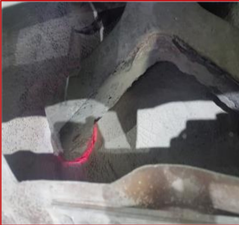
Red stub during preheat
