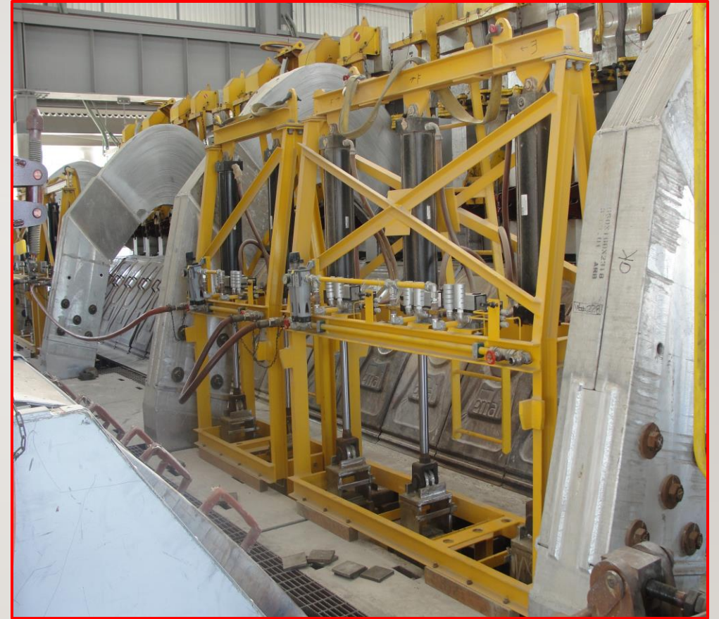
Short circuit wedge puller in place
