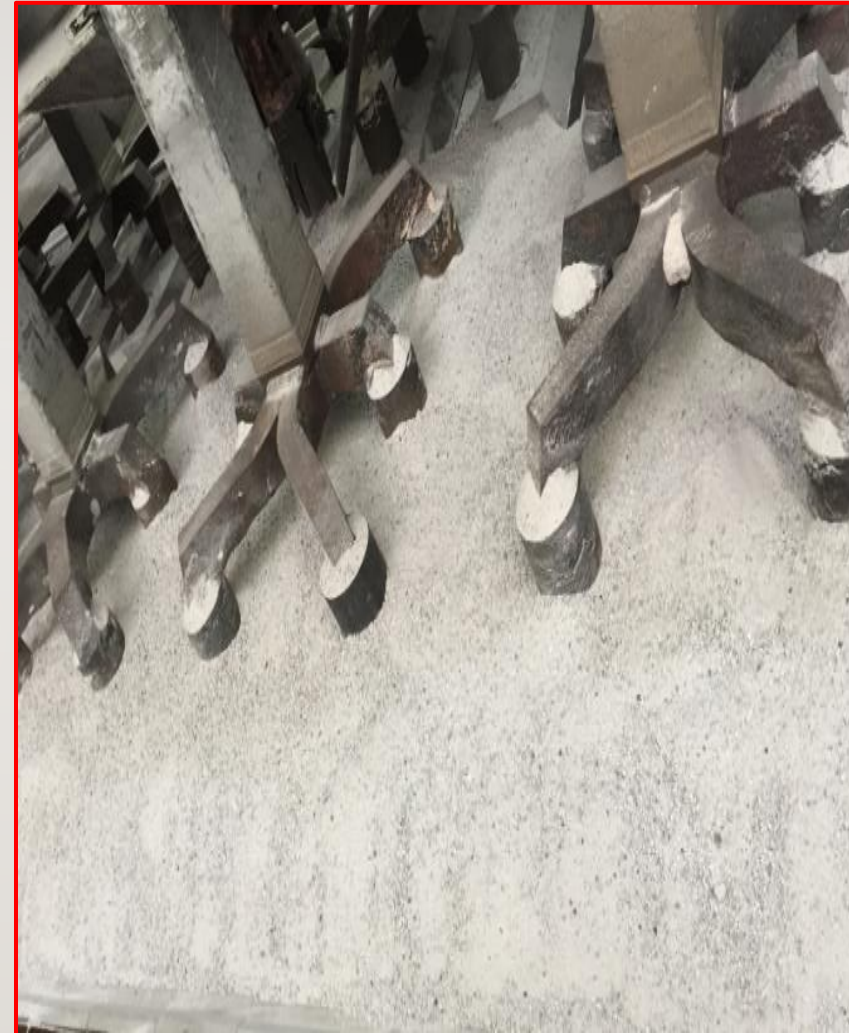
Anodes are well covered with crushed bath to avoid the heat losses
