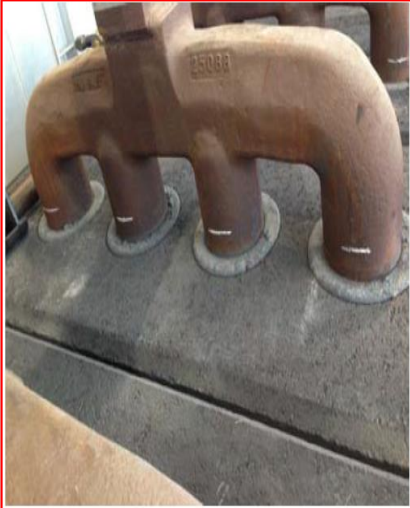
Anode stub marked with chalk to facilitate top covering
