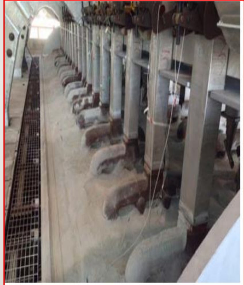
Anode top is covered with ACM
